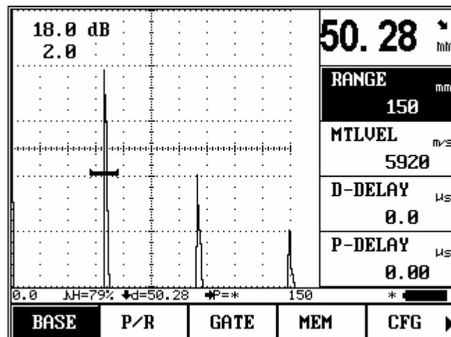
MTLVEL is unknown, set the approximate MTLVEL as 5920m/s, set the Gate Logic as double gate mode, meanwhile set the P delay as 0;
