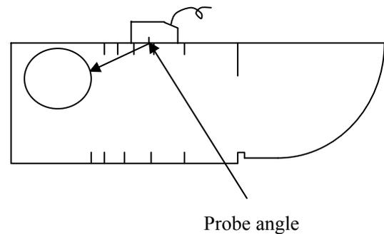
locate the probe as the right figure shows, move the probe back and forth to make sure you have got the highest echo, and now the scale corresponding with incidence point is the probe angle or K-Value.
