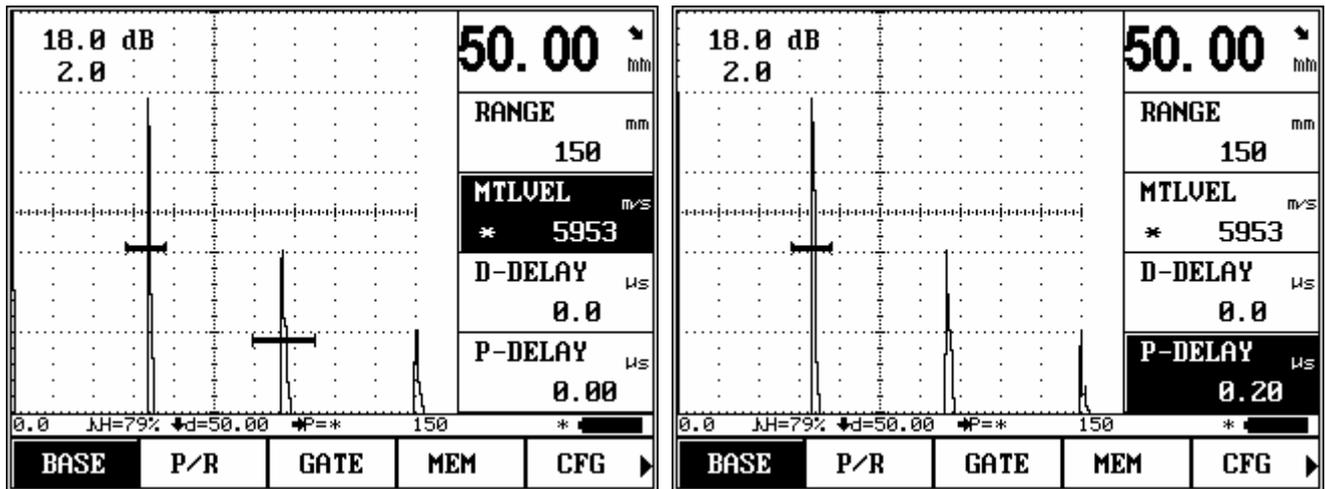
Increase MTLVEL, till the displayed pitch interval between the primary and secondary echo is 50mm, now we get the exact sound velocity of the material, i.e. 5953m/s;
