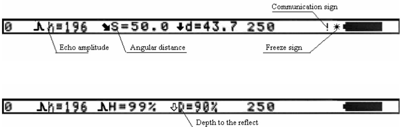
Fig. 3.9 Description about the display field in screen
