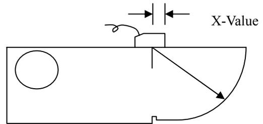
locate the probe on test block and move it as the right figure to make sure you have got the highest echo on R100mm reflector, measure the distance, which is the X-Value of probe, between the front face of probe and cycle center of R100m arc. The point corresponding to the cycle center of R100mm arc is just the incidence point of probe.
