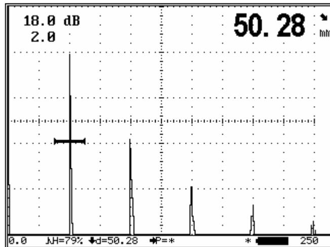
Fig. 3.8 A-scan at Enlarged mode
