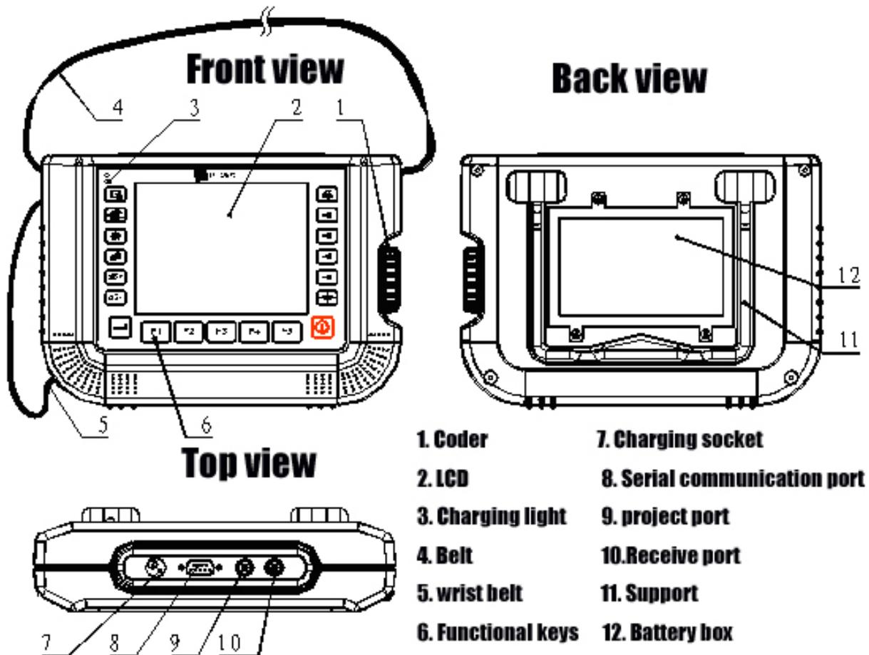
Fig. 3.1 Outside Drawing of the Instrument
