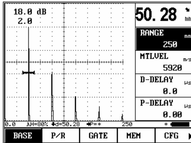
Fig. 3.7 A-scan at normal mode
