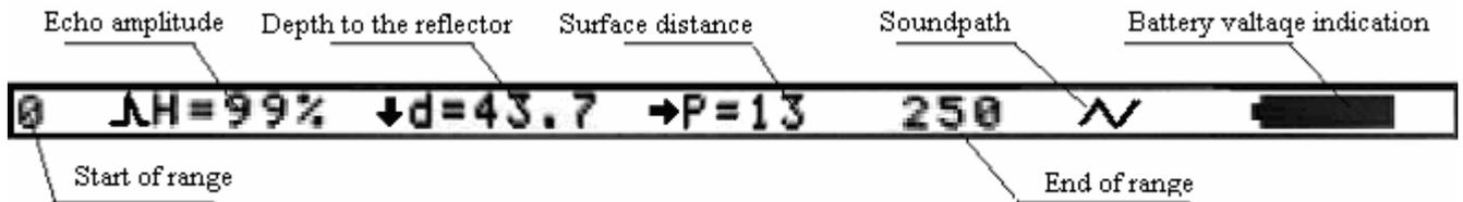
In the fig above, echo amplitude  $H=99\%$ , depth to the reflector  $=43.7\text{mm}$ , surface distance  $=13\text{mm}$ , echo times is 3, and battery voltage is high, start of range  $=0.0\text{mm}$ , end of range  $=250.0\text{mm}$
