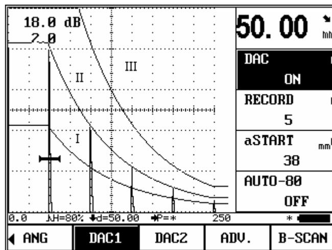
The screen is divided into three areas, I , II and III. The three curves will be drawn on the screen during the detecting, users can determine the flaw character by the height of the echoes.
